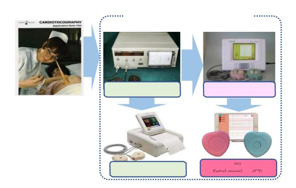
(Fig1) Fetal monitor weighed over 15 kg in 1970, whereas iCTG weighs about 300g, downsized to 1/50.
